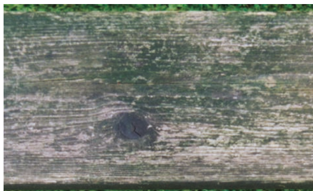
Treated Softwood in standard finish after 18 - 24 months
