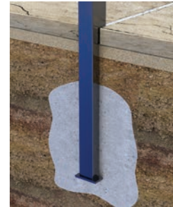
Extended leg, concreted in
